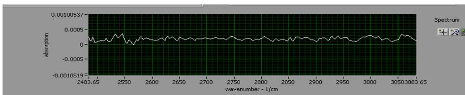
Figure 1. Baseline spectra, open beam, 500 scans
